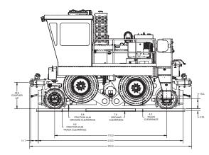
**Frame** Heavy-duty one-piece unitized frame welded from 3" steel plate.
