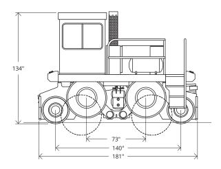
**Frame** Heavy-duty one piece, welded from 2" steel plate. Full width bumpers incorporates powertrain protection into design.
