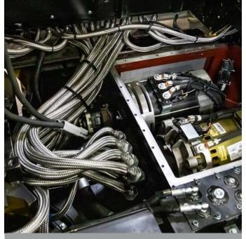
**FLEXIBLE CONDUIT (FC) CABLES** house regular cabling, which is sealed to ensure safe use in an EX-rated environment. The FC Cable provides flexibility and space saving.
