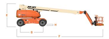
A. Platform Width 36-in / 91-cm B. Platform Length 96-in / 2.44-m C. Machine Width 8-ft 2-in / 2.49-m Tailswing 4-ft 8-in / 1.42-m E. Machine Height 9-ft 8.1-in / 2.95-m F. Machine Length 40-ft / 12.19-m G. Wheelbase 10-ft / 3.05-m H. Ground Clearance 11-in / 28-cm
