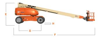
A. Platform Width 36-in / 91-cm B. Platform Length 96-in / 2.44-m C. Machine Width 8-ft 2-in / 2.49-m Tailswing 4-ft 8-in / 1.42-m E. Machine Height 9-ft 8.1-in / 2.95-m F. Machine Length 37-ft 6-in / 11.43-m G. Wheelbase 10-ft / 3.05-m H. Ground Clearance 11-in / 28-cm
