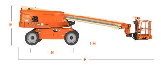
Platform Width 36-in / 0.91-m A. Platform Length 96-in / 2.44-m B. Machine Width C. 8-ft 2-in / 2.48-m D. Tailswing 4-ft / 1.22-m Ē. Machine Height 8-ft 2.4-in / 2.50-m F. Machine Length 28-ft 7-in / 8.71-m G. Wheelbase 8-ft 2.7-in / 2.5-m H. **Ground Clearance** 11.3-in / 29-cm
