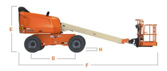
Platform Width 36-in / 0.91-m A. В. Platform Length 96-in / 2.44-m Machine Width 7-ft 6.8-in / 2.31-m D. Tailswing 2-ft 10-in / 86-cm Ē. Machine Height 8-ft 1.4-in / 2.47-m Machine Length Ē. 24-ft 11-in / 7.6-m Wheelbase G. 7-ft 9.5-in / 2.37-m **Ground Clearance** 12.1-in / 31-cm
