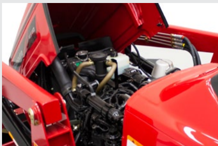
A one-piece steel hood provides easy access for maintenance work.
