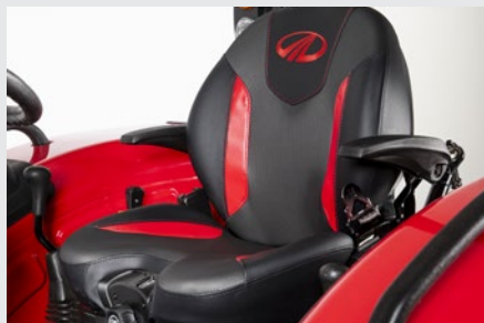
mComfort Mechanical Suspension Seat designed for maximum comfort and convenience, these mComfort seats come equipped with retractable seat belt, arm rests, and rainwater drain as standard.
