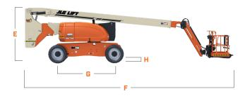
Platform Width 36-in / 0.91-m В. Platform Length 96-in / 2.44-m Machine Width 8-ft 1.5-in / 2.48-m C. Tailswing 2-ft 5-in / 74-cm D. E. Machine Height 9-ft 9.1-in / 2.97-m F. Machine Length 36-ft 9.9-in / 11.22-m G. Wheelbase 10-ft / 3.05-m **Ground Clearance** 11-in / 28-cm
