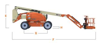
Platform Width 36-in / 0.91-m Platform Length B. 96-in / 2.44-m Machine Width 8-ft 2.2-in / 2.49-m Tailswing D. Zero Machine Height 8-ft 5.5-in / 2.58-m E. Machine Length 30-ft / 9.14-m F. Wheelbase 8-ft 1.9-in / 2.48-m **Ground Clearance** 11.8-in / 29-cm
