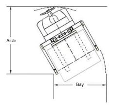
Note: Aisle dimensions listed above assume the bay width to be straddled OD plus 2" (1" on either side of straddle leg). Straddle OD is the load width plus 8". \*For metric conversion multiply inches by 25.4.
