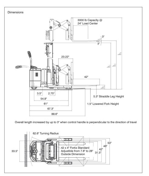
Note: Aisle dimensions listed above assume the minimum bay width to be straddle OD plus 5" (2.5" on each either side of straddle leg). Straddle OD is the load width plus 10". Truck performance may vary due to application requirements and changes in model design.
