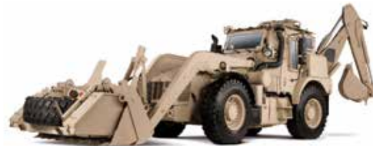
Built in Savannah, the fully armored JCB High Mobility Engineer Excavator (HMEE) is the world's toughest backhoe.
