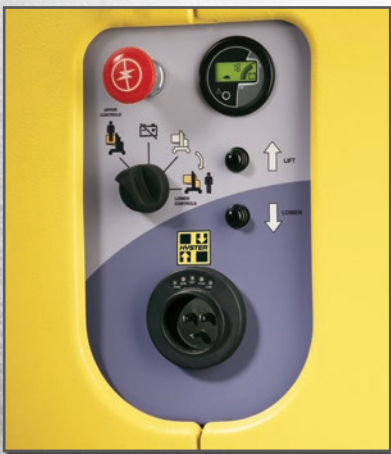
Lower control panel
