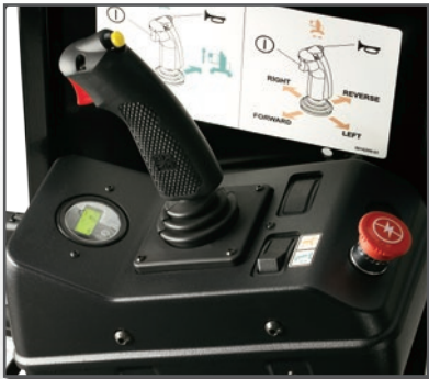
Upper controls with multifunction control handle
